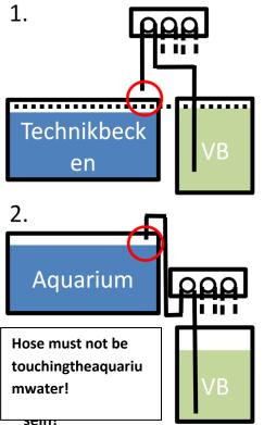
**Important:** The dosing pump and your outlets should always be above the top level of your Essential dosing solutions(1, 2 and 3). The outlet should also not be in contact with the aquarium water (red circle). The overall difference in heights should be minimal.
